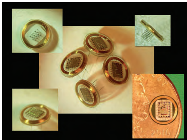
Figure. Miniature electrical stimulation modules that include up to 640 electrodes comprise the ICVP implant system.
