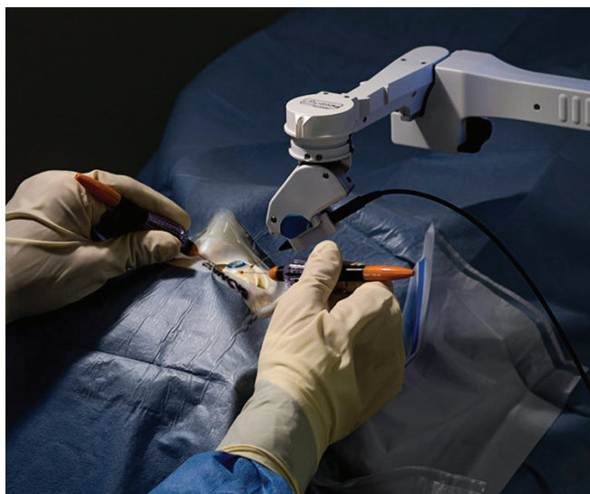
Figure 2. OOrimo, approved for use in Japan in 2023, uses a robotic arm to maneuver and stabilize an endoscope, allowing for bimanual surgery.
