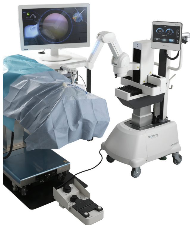
Figure. The surgeon operates the endoscope-holding robot using a foot switch while viewing the endoscope screen.
