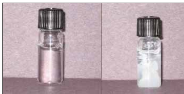
Figure 1. PNIPAAm is a thermoresponsive hydrogel. At room temperature it is a hydrated polymer that is hydrophilic in nature. With increase in temperature it collapses into a gel and becomes hydrophobic.
