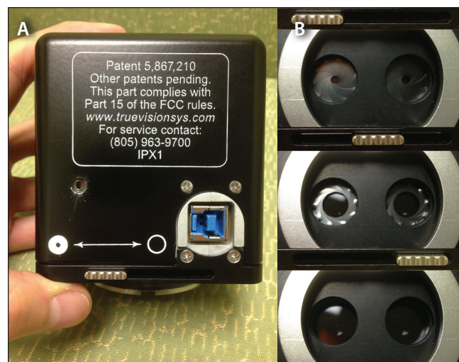
Figure 4. The Ngenuity camera (A). The sliding knob is used to adjust the iris aperture size. The iris apertures are on the bottom of the camera (B). The larger the aperture, the more light enters, but the depth of focus shallows. The smaller the aperture, the less light enters, but the depth of focus deepens. Having the iris open midway is a good place to start for vitrectomy cases. When switching to higher magnification for macular surgery, the iris can be slid further open so that endoillumination can be substantially lower. Because the range of focus required for macular surgery is small, the shallower depth of focus is not noticeable because one is operating well within that range with the full stereopsis provided by the Ngenuity system.
