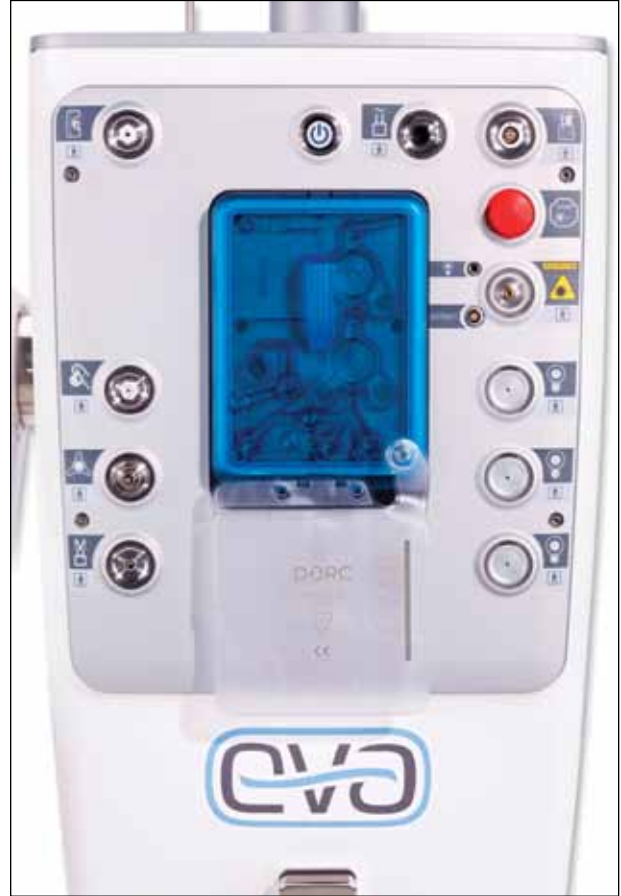
Figure 3. The 2 operating pistons and 3 closure valves. The operating pistons are situated over the micro-chambers. They operate in a synchronized manner and are constantly compensating changes in pressure, recognized by highly sensitive pressure sensors. Three closure valves, synchronized with the 2 operating pistons, allow the system to fill and empty the micro-chambers without any disruption in flow or pressure.
