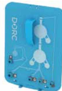
Front-loaded cartridge with color and form-coded connectors
