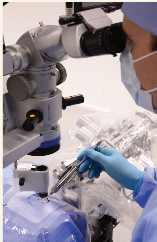
Figure 2. A robot arm steadies Dr. Stalmans' hand while he injects ocriplasmin into the occluded vein of a human patient with CRVO. Photo courtesy of UZ Leuven.
