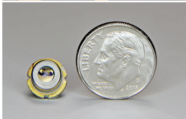
Figure 1. The laser source, half the size of a dime, is integrated into portable headset.
