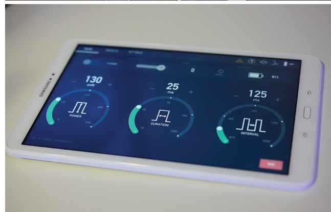
Figure 2. The Lion system is controlled with a user-friendly Android tablet and voice activation.
