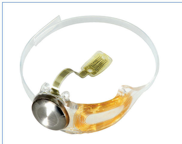
Figure 1. An illustration of the Argus II Retinal Prosthesis System showing the coil, cable, and electrode array.
