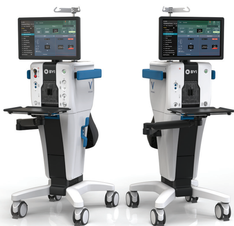
Figure 3. The Virtuoso DUAL combined phacovitrectomy machine, which has CE mark in Europe, is awaiting FDA approval.
