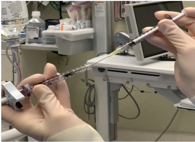
Figure 1. I load the therapeutic into the microinjector syringe through the front narrow end of the loading syringe to avoid air bubbles.
