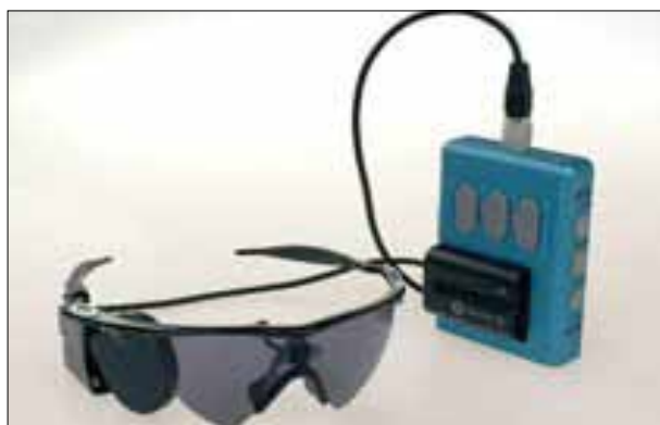
Figure 2. A miniature camera mounted on a pair of glasses is connected to an external video processing unit worn on the subject's belt.
