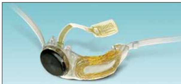
Figure 1. The Argus II system consists of a surgically implanted, 200- \mu m diameter, 60-electrode stimulating microelectrode array and an inductive coil link used to transmit power and data to the internal portion of the implant.
