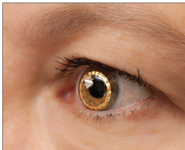
Figure 2. The Sensimed Triggerfish Sensor in the eye.
