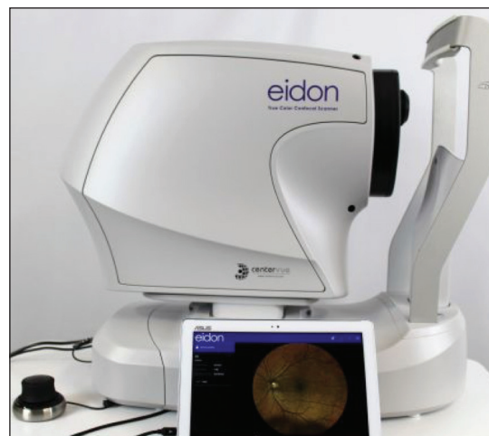
Figure 4. The Eidon fundus camera features an offset headrest design to minimize patient discomfort.
