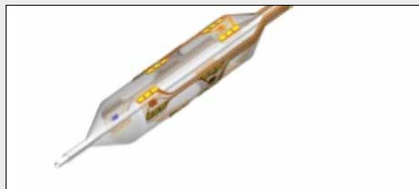
Figure 12. Close up of RF electrodes on balloon catheter.
