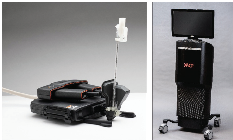
Figure 5. The platform of the Xact Ace robotic system is affixed to the patient and equipped with a motion sensor. Additionally, it features a flexible 5-DOF robotic arm with a needle holder and mobile monitor.
