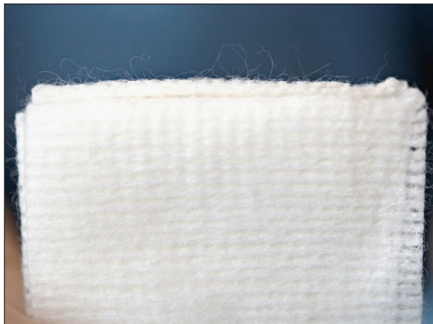
Figure 2. Cotton fiber shedding from the edge of a 4 X 4 gauze.
