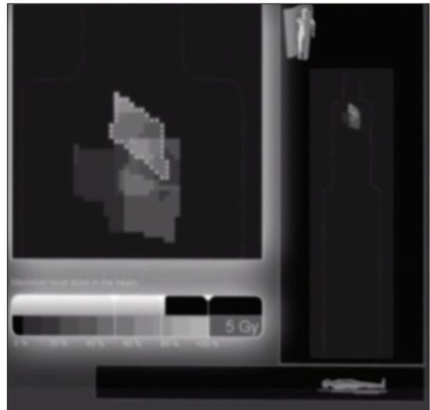
Figure 1. Dose map. Real-time visualization of cone beam projection and cumulated local dose.
