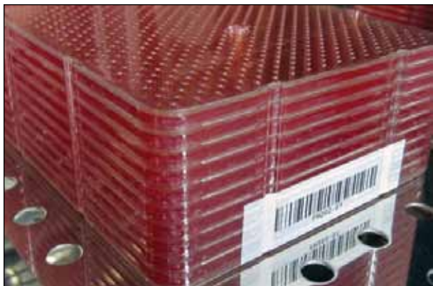
Figure 1. More effective cell amplification can be achieved by using modern cultureware options, such as this HyperFlask (Corning, Tewksbury MA), which uses approximately one-tenth of the space of traditional flask cultures.
