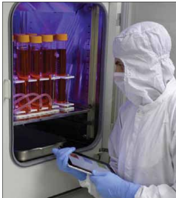
Figure 2. A compact bioreactor design will be key in producing tissue-engineered products at an acceptable cost. This system can typically support 60 vessels (up to 120) in 77 L of heated controlled atmosphere. The modular closed system provides both increased safety and ease of sampling for quality control.
