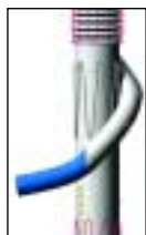
Figure 3. This diagram illustrates the helical wrap design for a branch-vessel device. The primary component has a limb that wraps around the tubular body at a given pitch such that it is appropriately oriented to the desired branch vessel. This is mated with a second stent graft (blue device) that can be trom-
