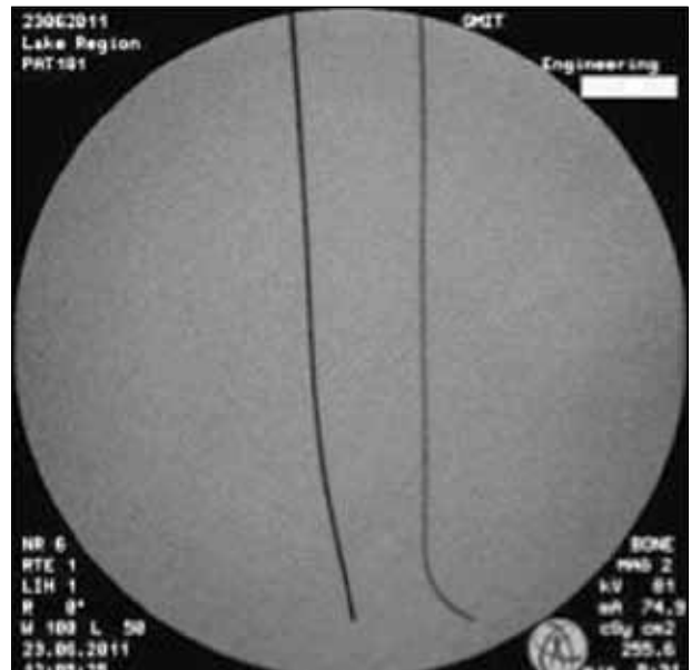
Figure 10. The same core diameter wire with different materials. Victory guidewire (Boston Scientific Corporation, Natick, MA) on the left.
