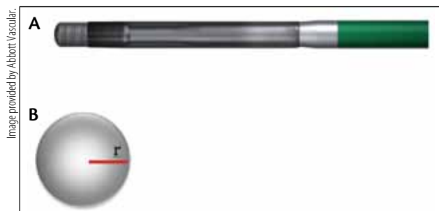
Figure 7. Measurements of tip penetration (A). Area of guidewire tip (B). Tip stiffness/area of guidewire tip: 0.004 kg/(3.14 X 0.006 inch 2 ). Penetration power = 40 kg/inch 2 .
