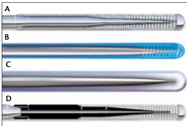
Figure 3. Stainless steel guidewires are generally easier to torque and provide better column support. The first-generation designs were made of just stainless steel (A), but the second generation upgraded to high-tensile-strength stainless steel (B). Nitinol guidewires are more flexible and kink resistant. The first generation of nitinol wires (C) were then enhanced by the second generation design of stainless steel and nitinol (D).
