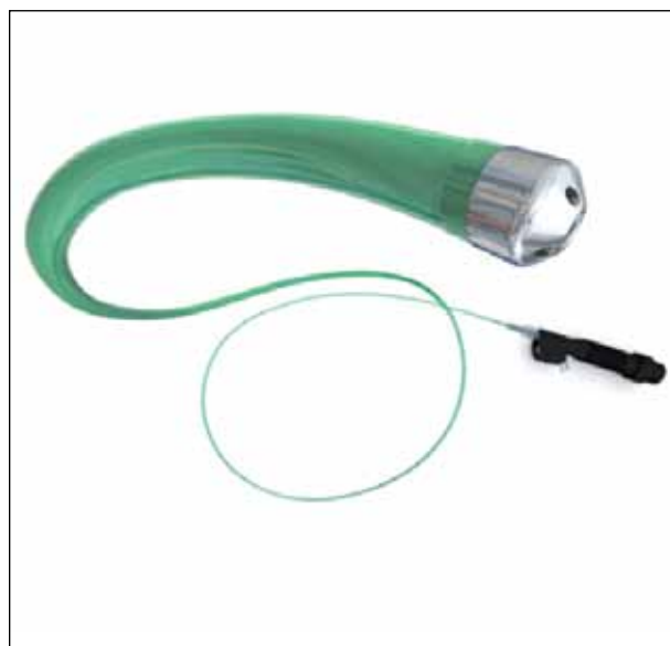
Figure 1. The Crosser catheter has a nitinol core wire that transmits mechanical vibration to the metal tip of the catheter at 20,000 cycles per second at 20- \mu m amplitude.
