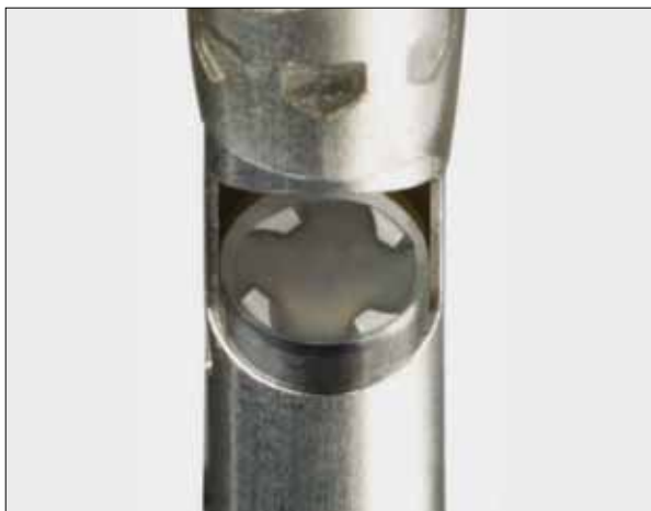
Figure 5. The calcium-cutting TurboHawk device (introduced in 2009) incorporates notches into the titanium-cutting blade that engages calcium more efficiently. Other enhancements include an improved fracture-resistant drive shaft and micro-efficient compression technology for improved compaction and capture efficiency of the excised plaque.
