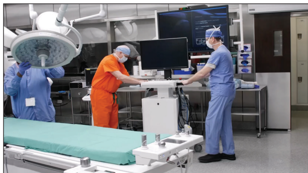
Figure 1. Separate mobile IOPS cart, which contains the interface and processor for guidance.
