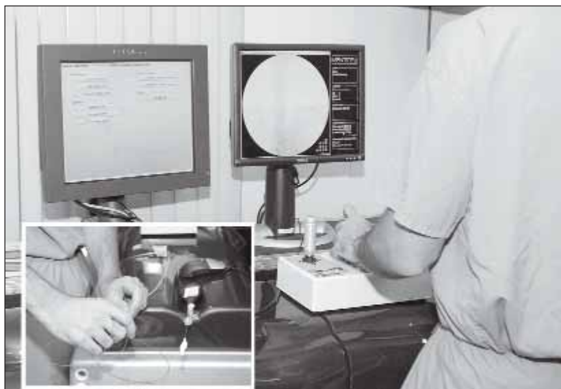
Figure 1. The ProCedicus VIST system. With a series of three haptic devices and specialized computer hardware, this endovascular simulator models the appearance of real-time digital subtraction angiography with computer-generated images responsive to actual hands-on catheter manipulation. Software packages include simulation for carotid artery disease, intracranial aneurysms, as well as coronary, renal, and iliac pathological conditions.
