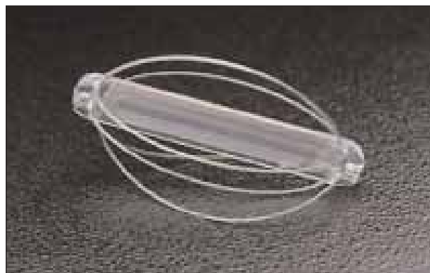
Figure 2. The EndoSure (CardioMEMS, Inc., Atlanta, GA) wireless pressure sensor.
