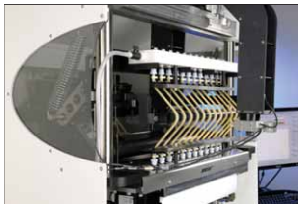
Figure 4. Testing device designed to apply bending forces. Systems capable of applying bending, such as this, offer improvements to designs that only cycle pressure. However, further improvements are required to better replicate the in vivo mechanical environment.
