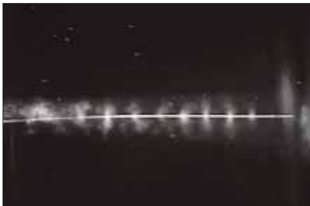
Figure 3. The OmniWave Endovascular System uses transverse ultrasonic energy to create cavitation streaming that rapidly resolves thrombus and quickly restores flow without adversely affecting surrounding structures. Longitudinal ultrasonic motion is converted to transverse motion along the treatment zone. Transverse micromotion creates stress waves to stimulate cavitation and streaming within the region of ultrasonic activation.
