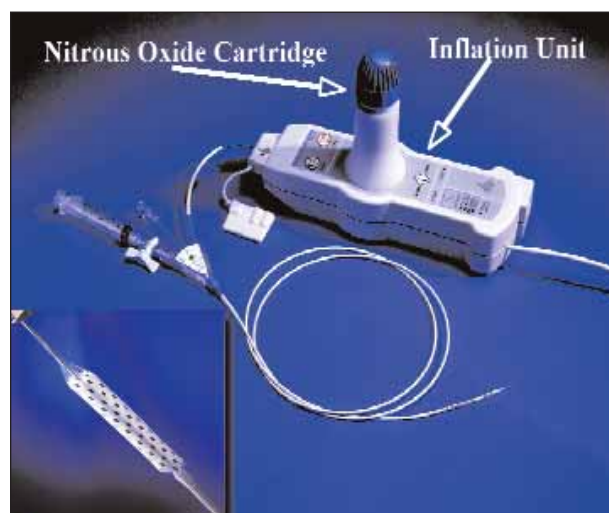
Figure 7. The PolarCath device (Boston Scientific Corporation). Cryoplasty uses nitrous oxide to inflate the angioplasty balloon to -10^{\circ}\text{C} with pressure of 8 atm for 20 seconds. The balloon with radiopaque markers (inset).
