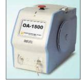
environment," co-owner David Centanni said. "In addition, the OA-1500 uses a standard SMA 905 universal connector, which makes it compatible with a variety of fibers, including reusable fibers."
