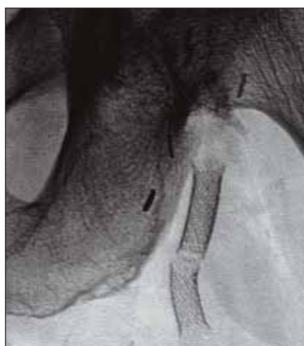
Figure 5. Radiograph showing complex fracture of a nitinol stent placed into a failing femoropopliteal bypass graft.
