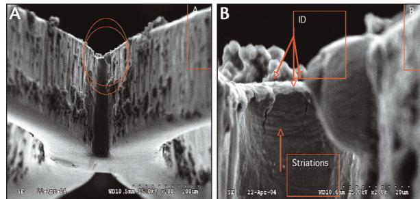
**Figure 2.** Scanning electron micrograph of a commercially available stent showing cracks, striations, and retained slag.
