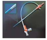
introducer sheath that can bend and flex without gapping, kinking, or producing sharp crimps, thereby minimizing potential trauma. According to the company, in benchtop tests, the Pinnacle TIF Tip required up to 24% less force in vascular entry than competitors' sheaths and, unlike comparative sheaths, flexed beyond 45° without kinking or collapsing. Reduced penetration force means the sheath is less likely to deform during vascular entry, resulting in easier, safer insertions, the company said.
