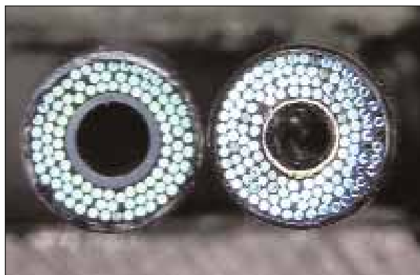
Figure 1. Features of the new 2.5-mm Turbo excimer laser catheter (right) compared to the 2.5-mm Extreme catheter (Spectranetics). Increased fiber density provides for greater energy delivery and better debulking.
