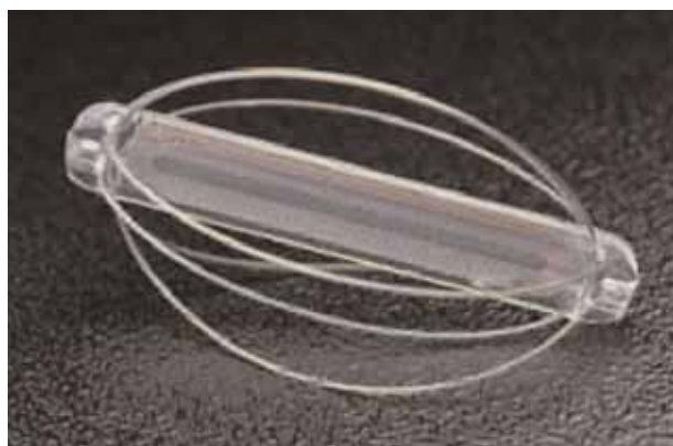
Figure 1. The CardioMEMS EndoSure Wireless AAA Pressure Sensor.
