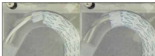
Figure 7. TX2 with Pro-Form with better accommodation of aortic arch curvature.
