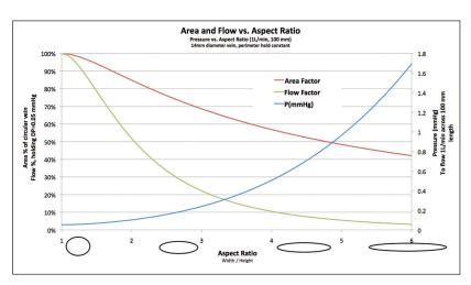
Figure 2. Holding perimeter constant, as the aspect ratio (ovality) increases, the area decreases. To maintain the same flow rate, pressure must increase.
