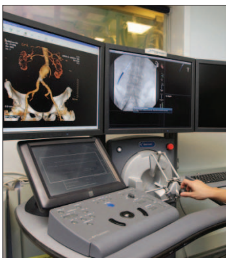
Figure 1. The Sensei robotic system (Hansen Medical, Mountain View, CA) workstation is shown outside the angiography suite during cannulation of the short contralateral limb of an infrarenal Endurant stent graft (Medtronic, Inc., Minneapolis, MN).
