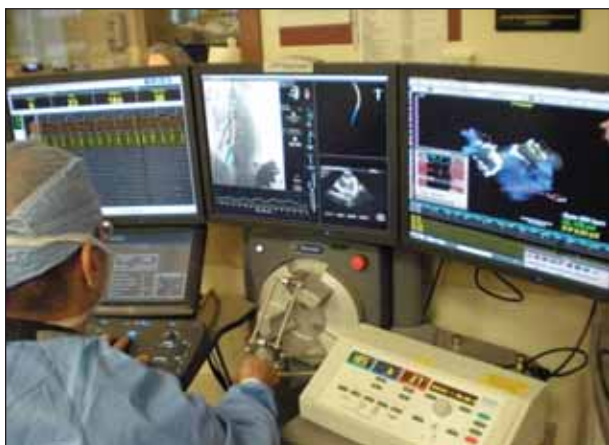
Figure 2. Virtual 3D rendering of the left atrium and virtual robotic catheter (Sensei System, Hansen Medical, Mountain View, CA) used for ablation of pulmonary vein orifices.
