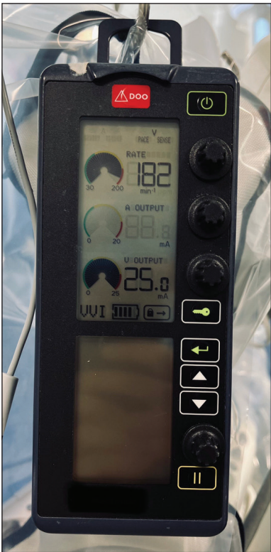
Figure 2. The external pacemaker programmed in VVI mode stimulating at 182 beats per minute with the maximum output energy (25 mA).
