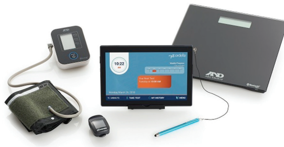
Figure 1. Cordella® HF System (tablet with patient app and Bluetooth®-enabled peripherals, including blood pressure, weight, heart rate, and SpO 2 ).
