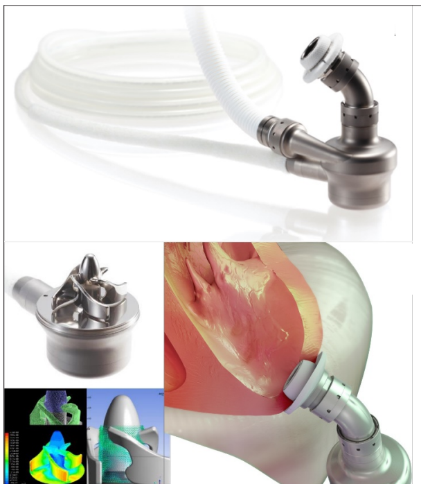
Figure 1. The Evaheart 2 device.
