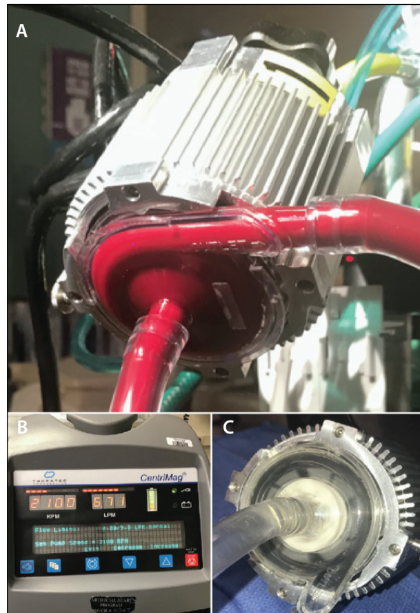
Figure 3. The CentriMag device with inlet from the patient and outlet to the patient (A). CentriMag is an optimal short-term RVAD that can achieve flows of up to 10 L/min (B). The levitating rotor ensures no frictional contact with the surrounding environment, which minimizes turbulent flow (C).
